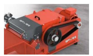
Powerful and low-maintenance drive via electric motor and V-belt
